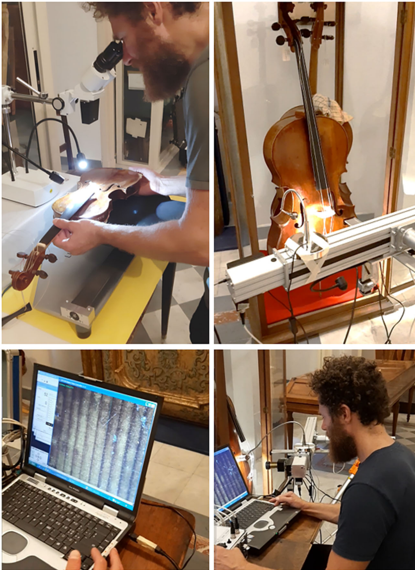
FIGURE 1 Sampling practices: (top left) portable dendrochronograph with stereomicroscope. The other images refer to the video time table (VTT) during the measurement of the tree-rings on a cello without removing the instrument from its case.
